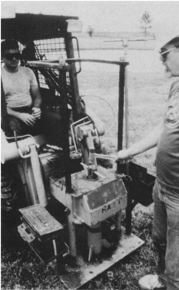
FIG. 2. The 8-gauge Auger gun with Case 1825 skid steer loader.
