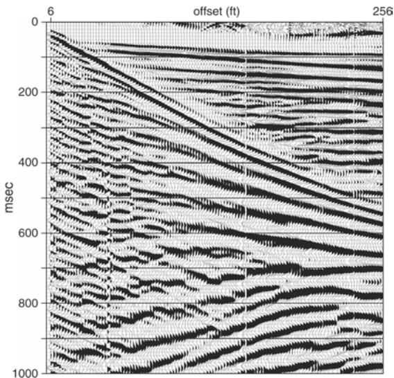
Figure 2. AGC (automatic gain control) applied to the raw vibroseis record. With all the coherent arrivals amplitude enhanced.
