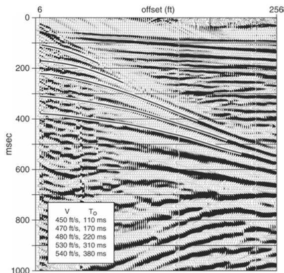
Figure 4. NMO velocity curves superimposed on the shot record.
