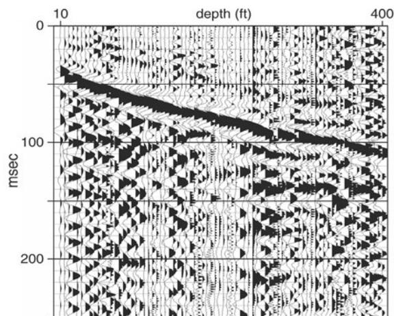
Figure 5. Shear wave down-hole survey. The high velocity bedrock at around 3 m depth is a clear indicator that the extremely low NMO velocities observed in arrivals within the noise cone are not realistic for this site.
