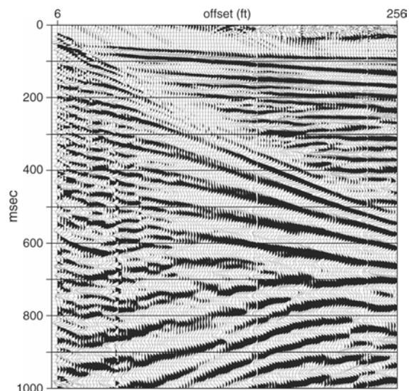
Figure 3. F-k filtering reduces or eliminates the linear arriving surface wave and enhances the curved arrivals within the noise cone.
