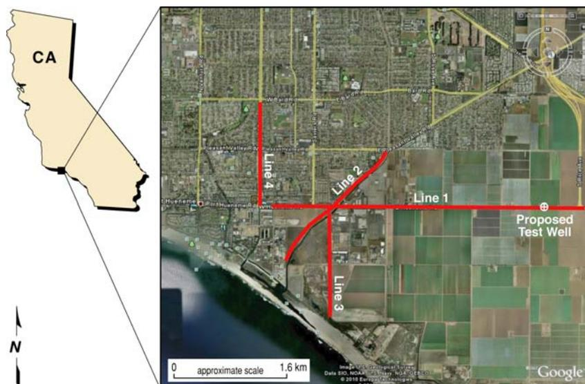
Figure 1. Site map with four seismic lines highlighted in red. Line 4 was acquired in a dry cement drainage canal.
