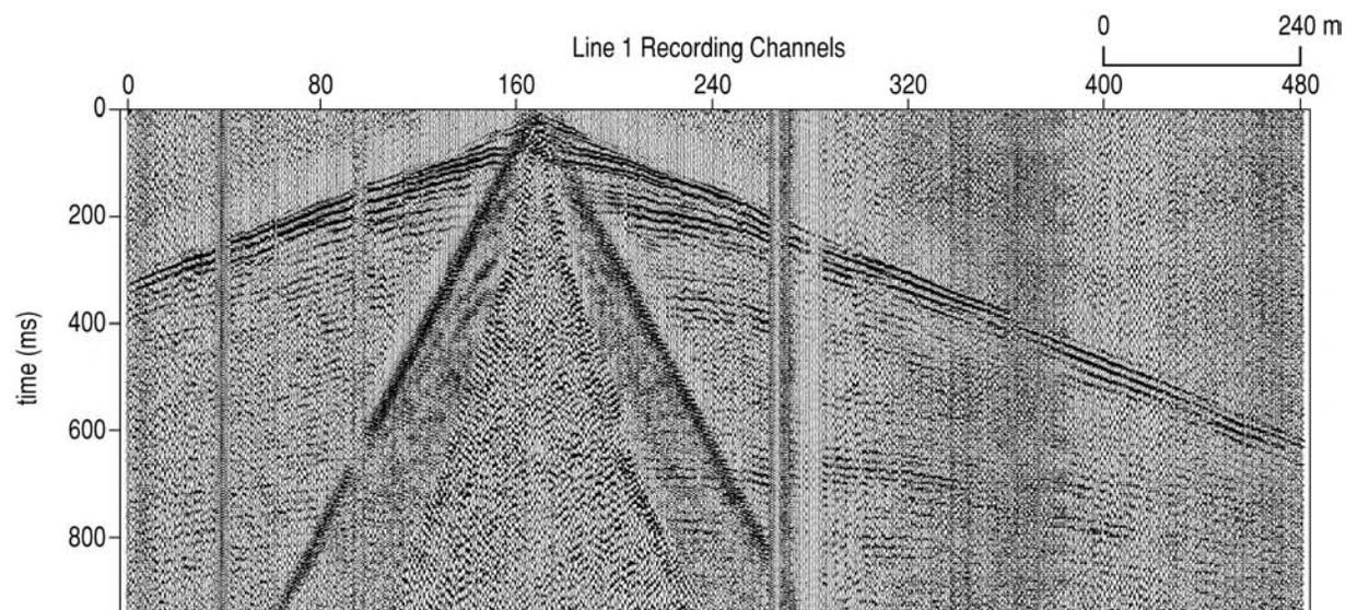
Figure 3. Correlated shot gather from line 1 (Figure 2) with dead traces from road intersections obvious. Most vehicle and power line noise suppressed near background levels. Recording channel 160 correlates to CMP station 1300 on CMP stacked section (Figure 4).
