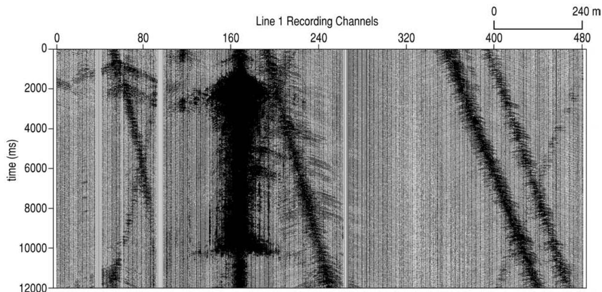
Figure 2. Uncorrelated 12-second sweep with traffic noise obvious. Power lines cross the profile near channel 300. All dead traces are the result of road crossings. Recording channel 160 correlates to station 1300 on CMP stacked section (Figure 4).
