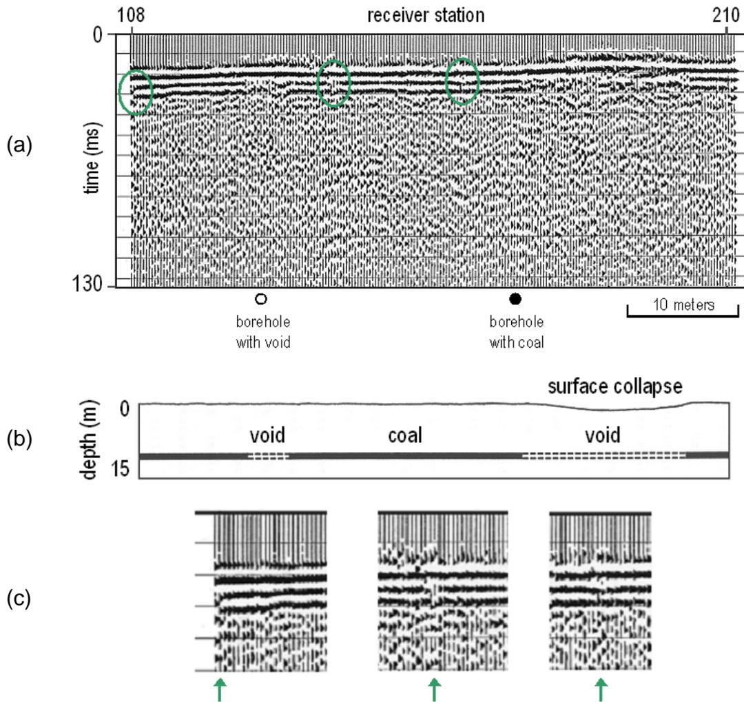
Figure 1: (a) Seismic profile and (b) interpreted cross-section resulting from standard CMP processing. Green circles in (a) indicate subtle discontinuities in the reflection from the top of the coal that are not associated with the interpreted voids. (c) Close-ups of the discontinuities in (a) indicated with an arrow. Modified from Branham and Steeples (1988).
