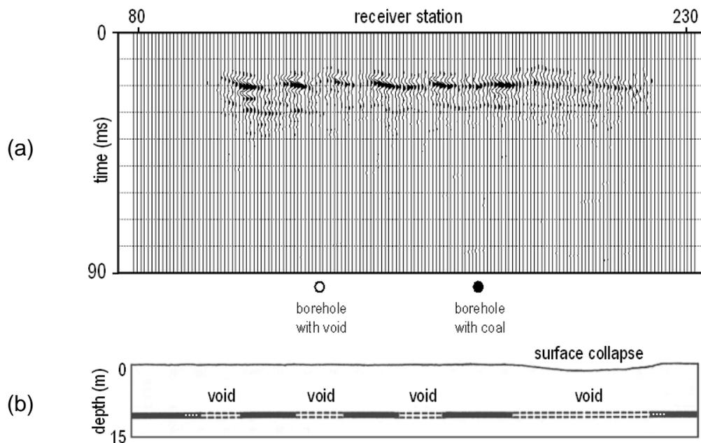
Figure 2: (a) Seismic profile and (b) interpreted cross-section resulting from the diffraction imaging algorithm.
