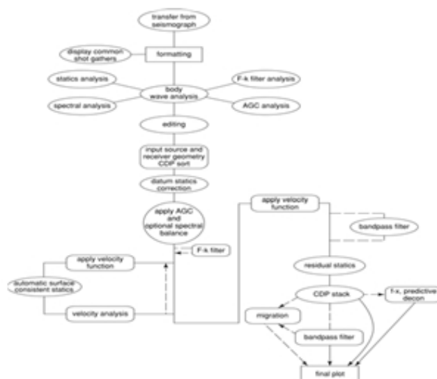
Figure 3: CMP processing flow used for these data flow. Pre-stack is any process before CDP stacking.
