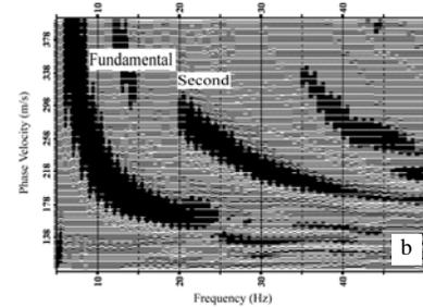
Figure 1. An example from San Jose, California (Xia et al., 2003). a) Raw surface-wave data and b) their image in the frequency-velocity domain.
