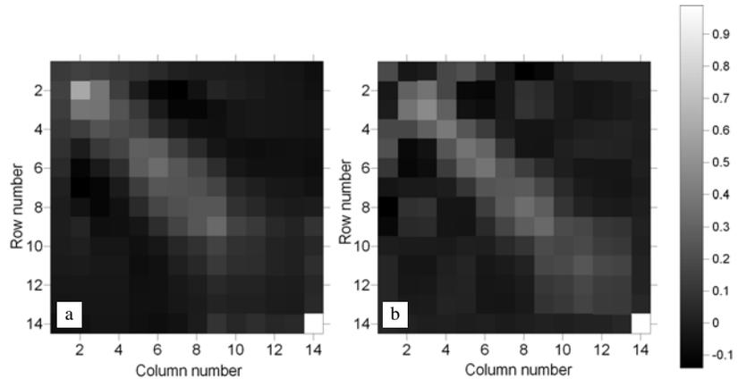
Figure 4. The model resolution matrixes of the San Jose example (Xia et al., 2003) based on a) the inverted model from 28 data and on b) the inverted model from 16 selected data associated with the corresponding diagonal values of the data resolution matrix of 0.45 and higher.
