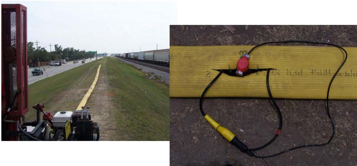
**Figure 2:** (a) Accelerated weight-drop seismic source and land streamer used for the MASW survey, Citrus Lakefront Levee, New Orleans, Louisiana. (b) Close-up of 4.5-hertz vertical displacement geophone housed within the land streamer.
