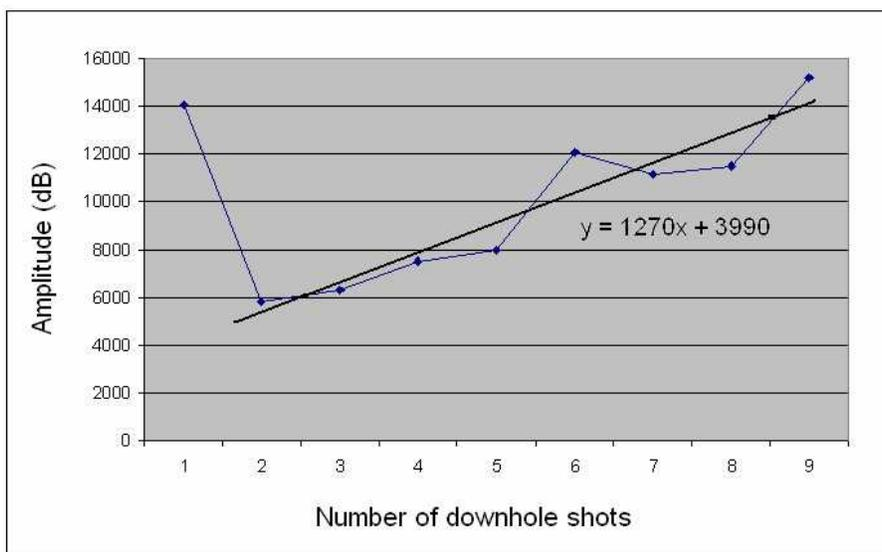
**Figure 1** – Average change in air-coupled wave amplitude. There is a 59% amplitude decrease between one and two downhole shots, followed by a nearly linear amplitude increase for the remaining shots.
