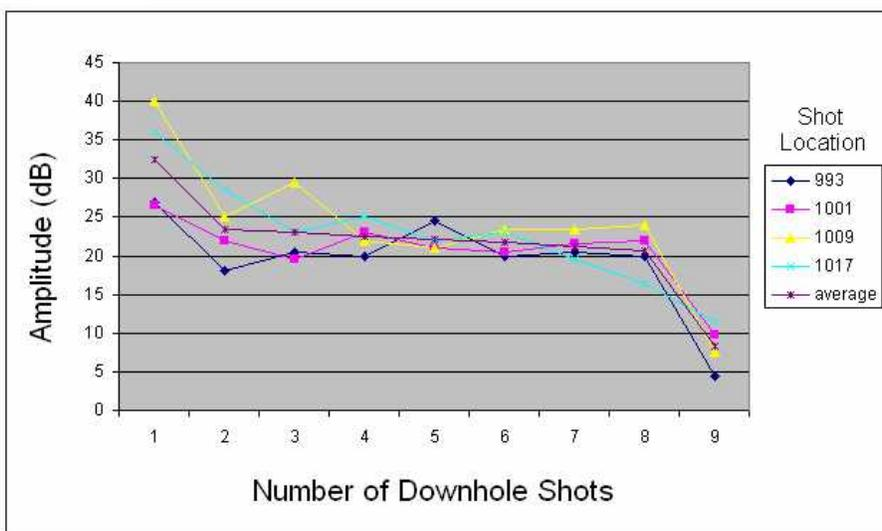
**Figure 2** – Change in absolute reflection amplitude as a function of number of downhole shots fired for the 55 ms reflection in four shot gathers.
