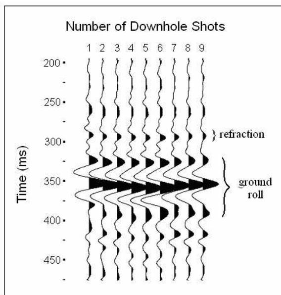
**Figure 6** – Nine traces corresponding to the same shot (1017) and receiver (1120) station for each survey. The refracted energy arrives at approximately the same time. Ground roll traveltime appears to change as shots are fired downhole.
