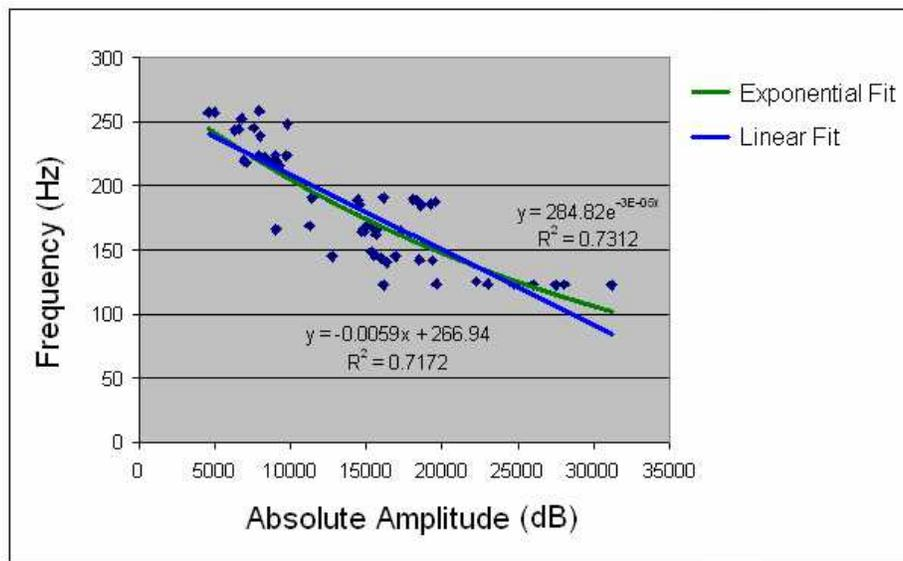
**Figure 4** – The average frequency versus amplitude of unmuted data.
