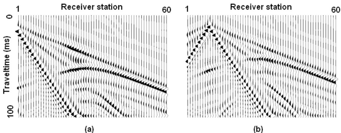
Figure 2: Bandpass filtered synthetic shot gathers containing diffraction hyperbola, caused by the tunnel. The source in (a) is at station 1000; the source in (b) is at station 1010. The apex of the hyperbola is laterally located at the same station in both gathers.
