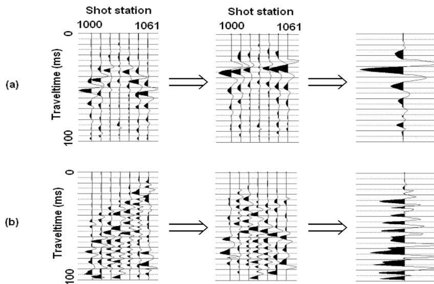
Figure 4: Common receivers prior and subsequent to normal moveout correction, and resulting stacked trace. (a) The common receiver gather for the receiver above the tunnel contains a diffraction hyperbola that is properly moved out and horizontally stacked, resulting in a large-amplitude wavelet. (b) The common receiver gather for the receiver at station 1060 contains no visible diffraction hyperbola, does not flatten, and results in a noisy trace.
