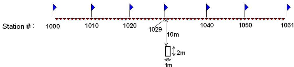
Figure 1: Model fixed receiver spread configuration above a tunnel. Receiver spacing (receiver stations are denoted by a red triangle) is 1 m, source spacing (source stations are denoted by a blue flag) is  $10 \pm 1$  m. The  $2 \times 1$  m tunnel is located 10 m beneath the midpoint between stations 1029 and 1030.
