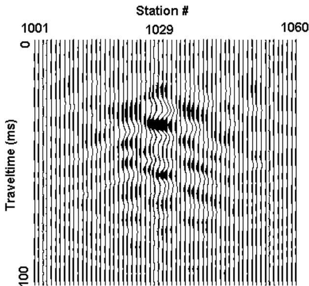
Figure 5: Resulting traces from NMO correction and horizontal stacking in the receiver domain. The relatively large-amplitude wavelets resulting from the tunnel are clearly visible on traces corresponding to stations 1027 through 1032 at roughly 24 ms, the time corresponding to the shortest two-way traveltime when the source was directly over the tunnel.
