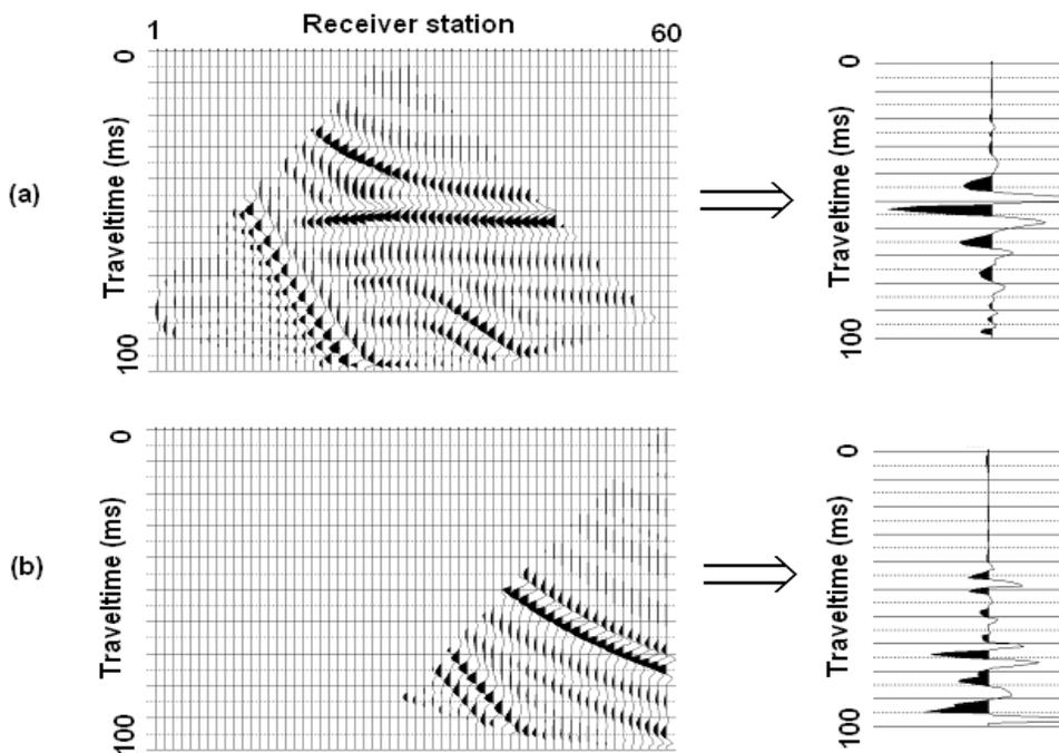
Figure 3: NMO corrected duplicate shot gathers associated with source station 1000, and resulting traces after horizontal stacking. The source was assigned to station 1029 in (a) and station 1060 (b). Only the traces in gather (a) properly moved out and flattened, resulting in a high-amplitude wavelet.
