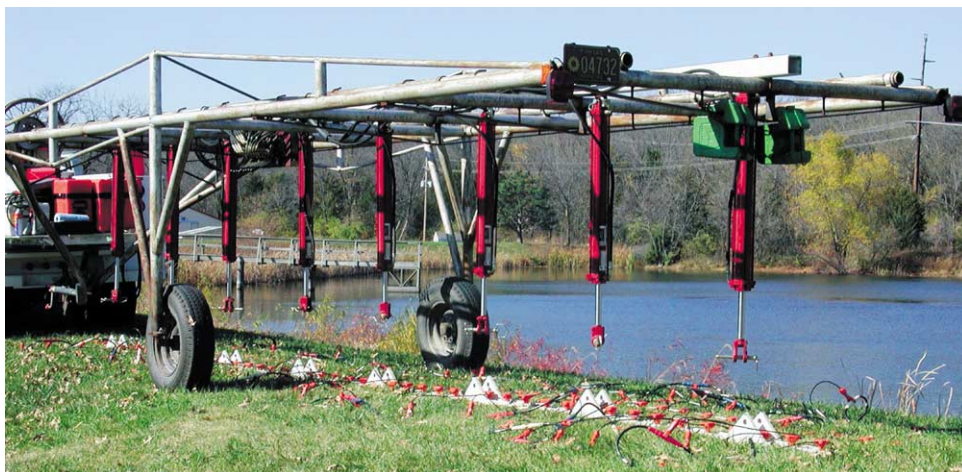
Fig. 1. A photo of the autojuggie field layout with the hydraulic cylinders detached from the steel bars to which the geophones are rigidly bolted.
