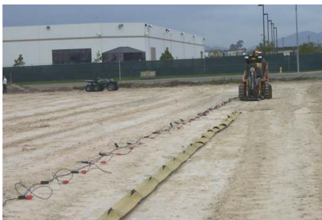
Figure 5: Equivalent source energy was recorded by both receiver spreads here at the San Diego site and at the KS/OK site.
