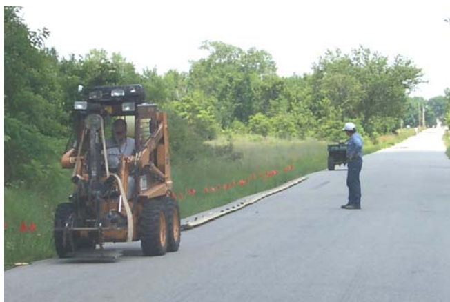
Figure 3: The towed array is pulled by a self-propelled weight drop style seismic source. The spread is attached to the source vehicle by an electric winch, providing real time offset adjustments and the option to decouple the source and spread by letting the cable go slack.
