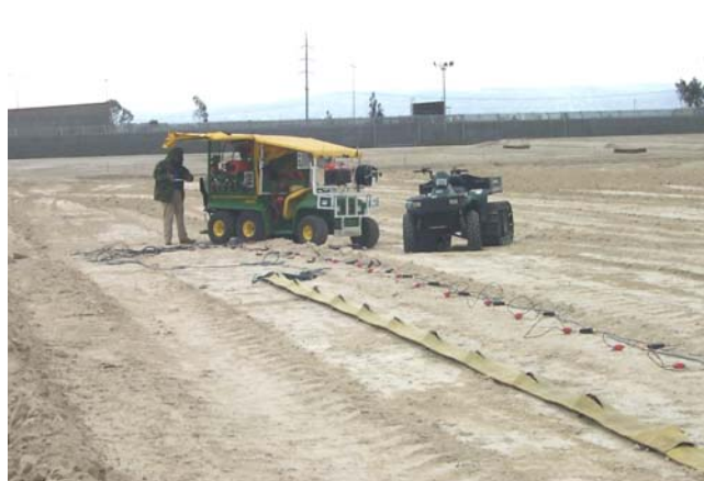
Figure 4: Comparison of spike planted geophones and the towed spread geophones at the San Diego, California, site was ideal since the ground had just been worked uniform in preparation for construction of a commercial building.
