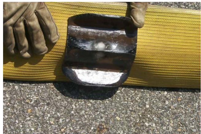
Figure 2: Inside the fire hose the two geophones (one shear and one compressional) are mounted to a steel plate attached to the bottom of the fire hose and representing the ground contact/coupling. The aggressive design of the outrigger style contact provides level support on paved surfaces and a cutting action in soils or light vegetation.
