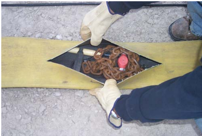
Figure 1: Top view of towed array. A surplus fire hose is used to enclose the receivers and cable, maintain spacing between receivers, and provide the tow line.
