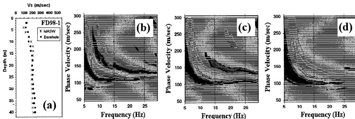
Figure 4. (a) Down-hole  $V_s$  profile for FD98-1 well and multimodal dispersion curve analysis for three shot records obtained with source-to-nearest receiver distance of (b) 17.1m, (c) 8.5 m, and (d) 2.4 m.
