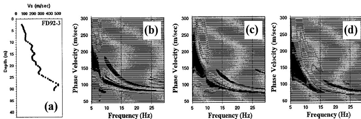
Figure 5. (a) Down-hole  $V_s$  profile for FD92-3 well and multimodal dispersion curve analysis for three shot records obtained with source-to-nearest receiver distance of (b) 17.1m, (c) 8.5 m, and (d) 2.4 m.
