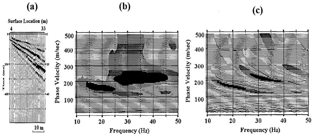
Figure 2. (a) A 30-channel shot record collected at a Geometrics test site, San Jose, California. A 20-lb hammer and 4.5-Hz geophone were used as source and receivers, respectively. (b) Result of multimodal dispersion curve analysis from the conventional method ( $\tau - p$  transformation) (McMechan and Yedlin, 1981). (c) Same type of result from the new transformation method by Park et al. (1998b).
