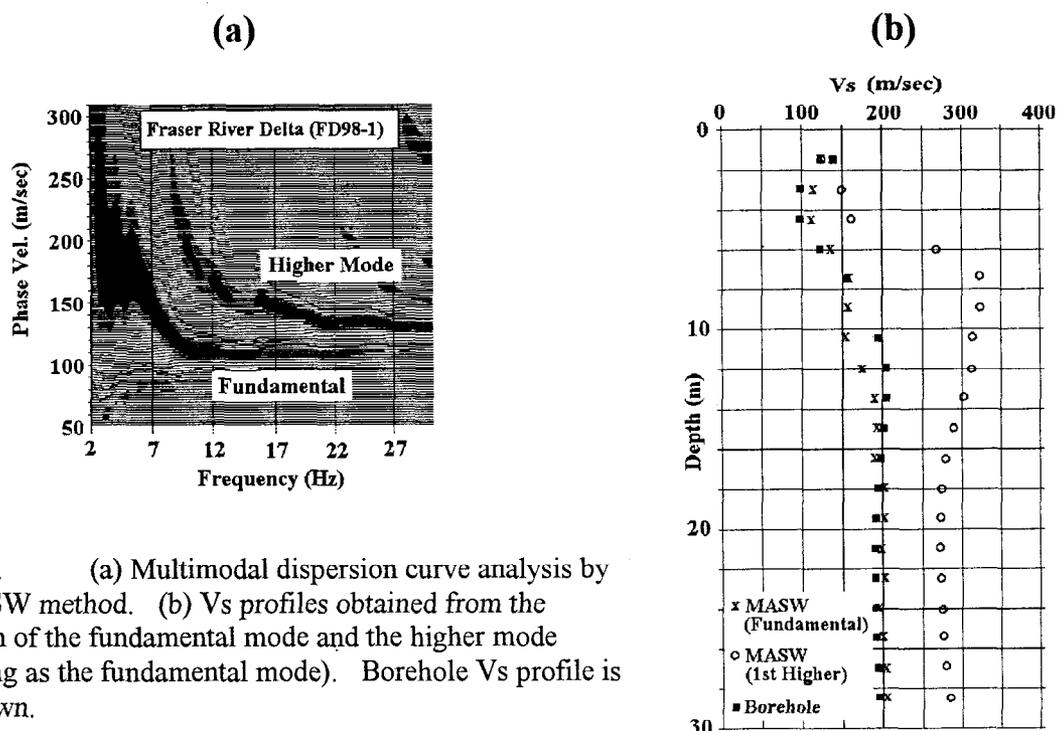
Figure 1. (a) Multimodal dispersion curve analysis by the MASW method. (b)  $V_s$  profiles obtained from the inversion of the fundamental mode and the higher mode (assuming as the fundamental mode). Borehole  $V_s$  profile is also shown.
