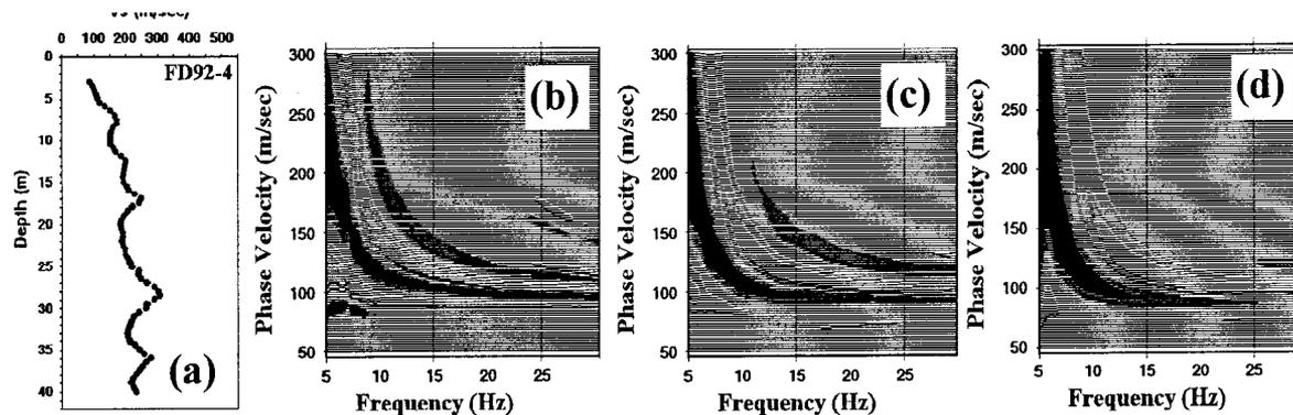
Figure 6. (a) Down-hole  $V_s$  profile for FD92-4 well and multimodal dispersion curve analysis for three shot records obtained with source-to-nearest receiver distance of (b) 17.1m, (c) 8.5 m, and (d) 2.4 m.
