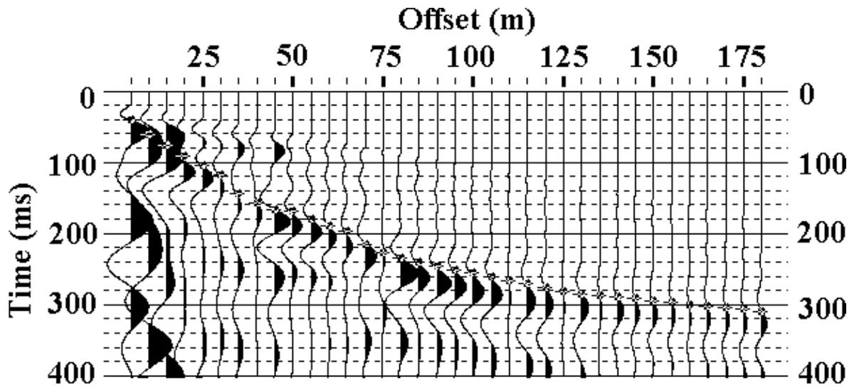
Figure 3. Refraction inversion using 70 m deep velocity model.
