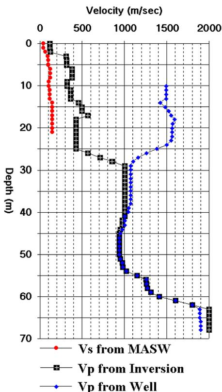
Figure 4.  $V_s$  profile from surface (Scholte) wave inversion and  $V_p$  profile from well and refraction inversion.
