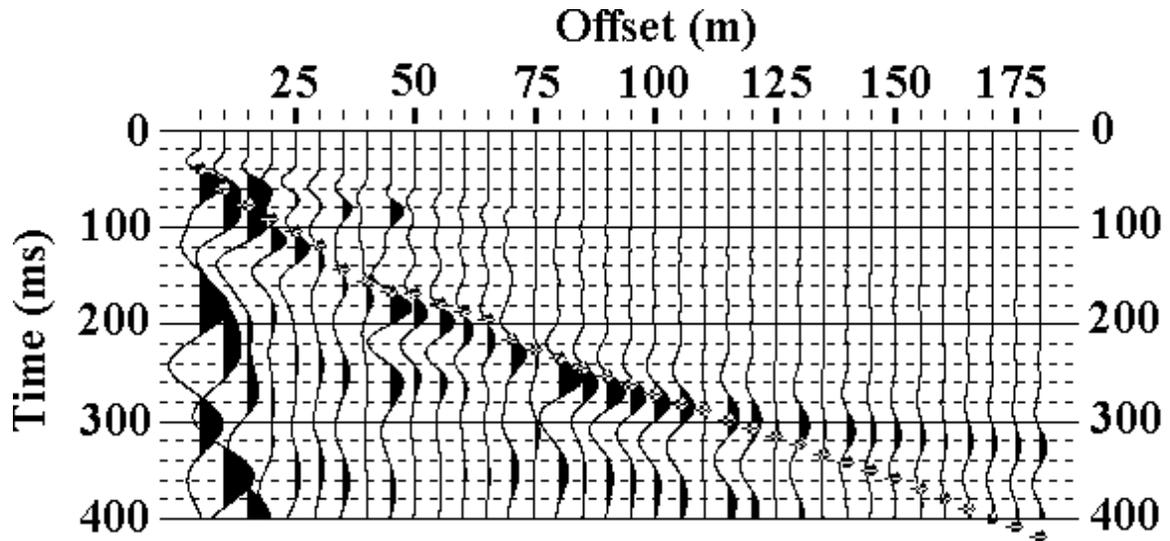
Figure 2. Refraction inversion using only 21 m deep velocity model.
