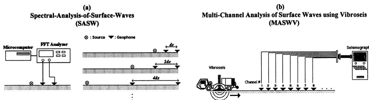
Figure 1. Basic configurations of (a) Spectral Analysis of Surface Waves (SASW) and (b) Multi-channel analysis of surface waves using Vibroseis (MASWV) methods.
