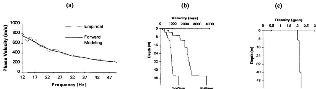
Figure 3. (a) Dispersion curves from acquired data (empirical) and forward modeling, (b) velocity, and (c) density models used for the forward modeling.
