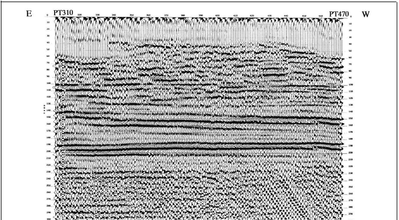
Figure 2. 24-fold CMP stack of pre-test data collected with an auger gun source before the non-invasive source test. Many shallow reflectors appear above the dominant 160ms and 200ms reflectors. CMP spacing is 0.6m (2 feet).
