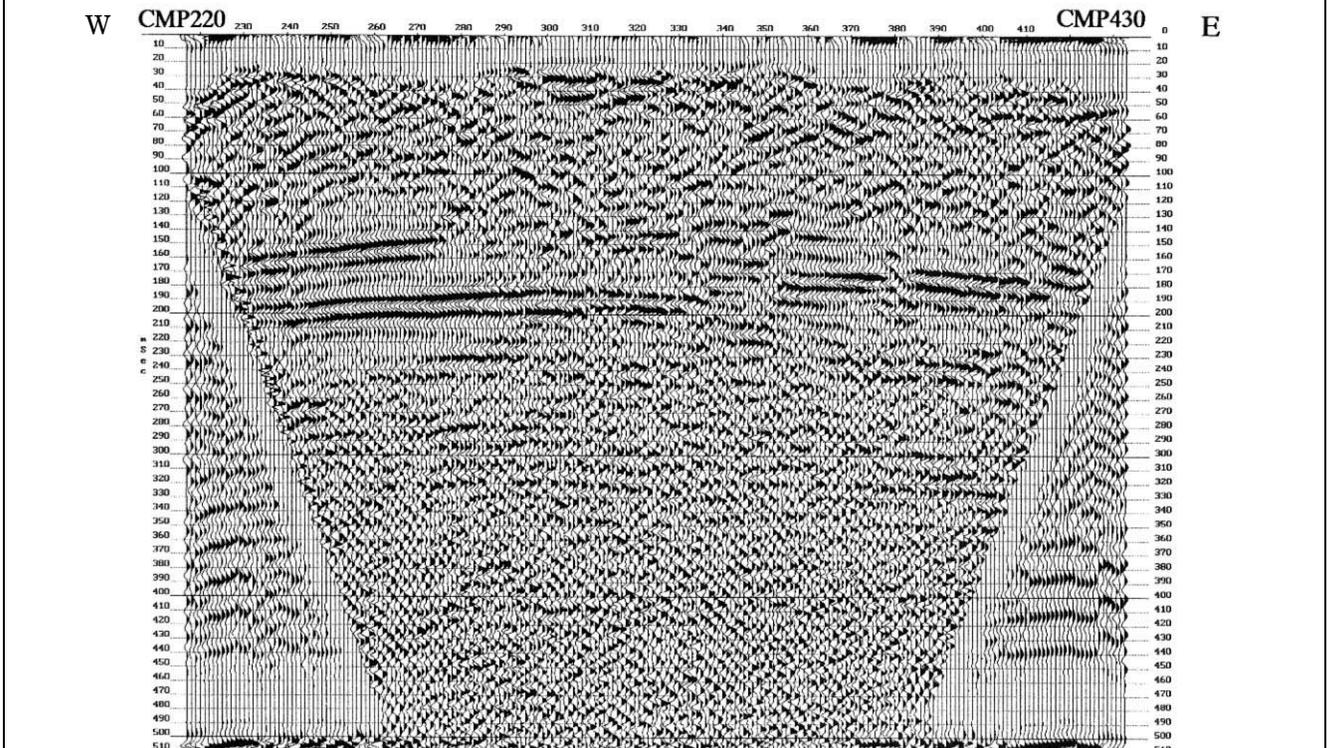
Figure 3. Brute stack of up to 66-fold CMP data from the non-invasive source test. Stacking of large offset data appears to degrade shallow reflectors.
